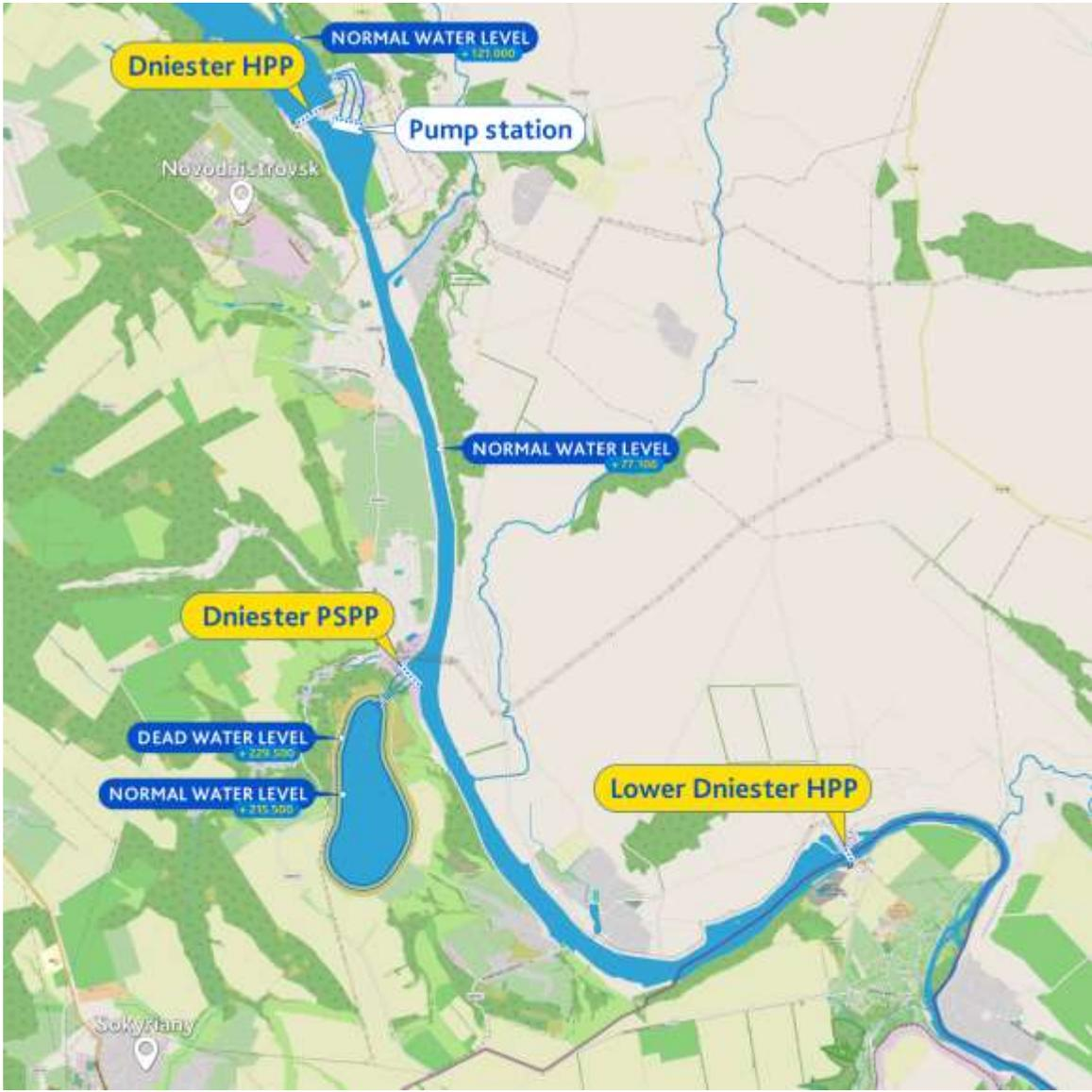
The main facilities of the pumping station are located on the left bank of the Dniester River, at the upper and lower reaches of the Dniester HPP dam. The water intake is located on the bank of the Dniester reservoir. The pumping station building is located in the Lower Dniester Reservoir. The pressure tunnels are in the rock mass at +58.600 to +59.695 meters.
