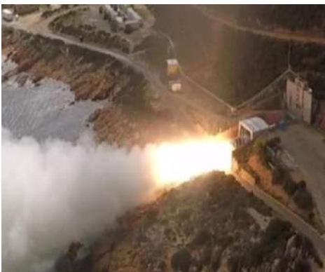
Z40 Static Firing Test (March 2018, Sardinia)
